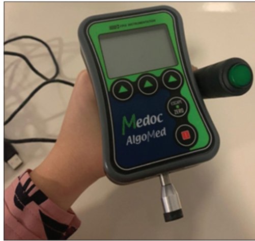
Supplementary Figure 1: Algomed device for quantitative sensory testing.
