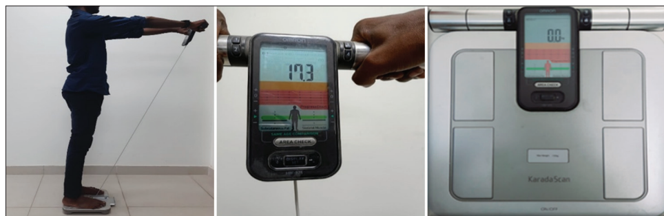
Figure 3: Measurement of body composition with the help of a bioelectrical impedance analyser.
