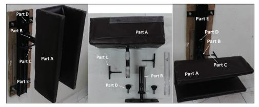
Figure 1: Elbow isometric exercise instrument, a custom-made instrument for performing elbow flexors and extensors isometric exercise at different elbow joint angles. Part E is fixed to a wall.
