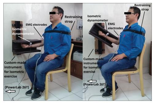
Figure 2: Experimental set-up for data recording of isometric elbow flexors and extensors strength curve.
