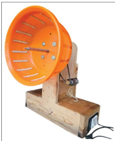
Figure 4: Full view of the motorized rodent wheel.
