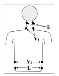
**Figure 2:** Placement of electrodes  $(I_1, I_2, V_1, and V_2)$  on the body surface for the determination of cardiac output.
